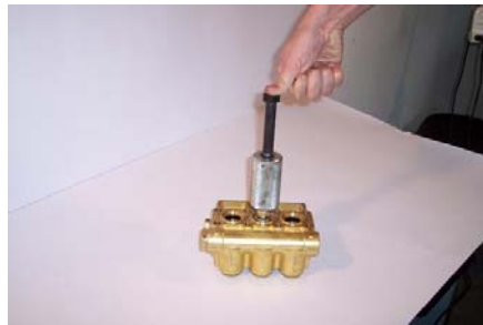
Insert the drawer in the plunger's seat
