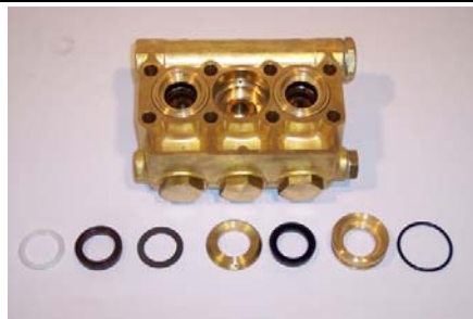
Unscrew the drawer and take out the seals package
