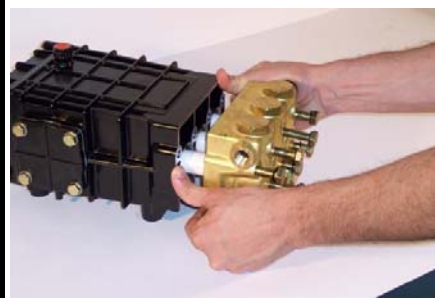
Remove the head from plungers
