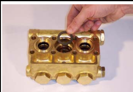
Insert the washer in the plunger's seat
