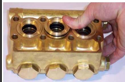
Push the back brass ring in the plunger's seat
