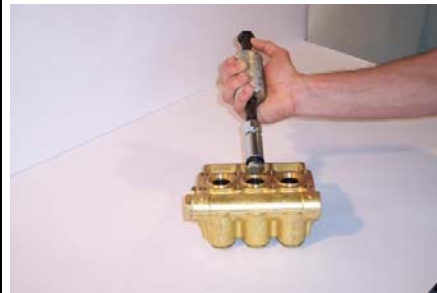
Insert the drawer in the plunger's seat
