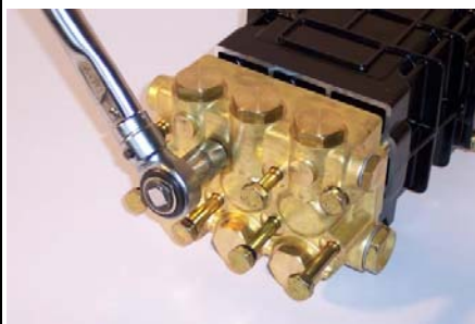
Turn out the screws that clamp head with crankcase
