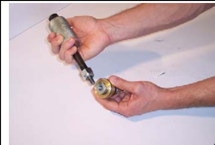
Unscrew the drawer and take out the seals package
