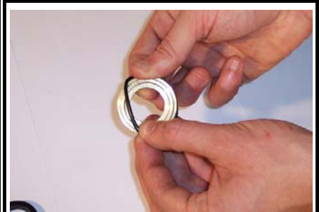
Slip the OR on the back brass ring
