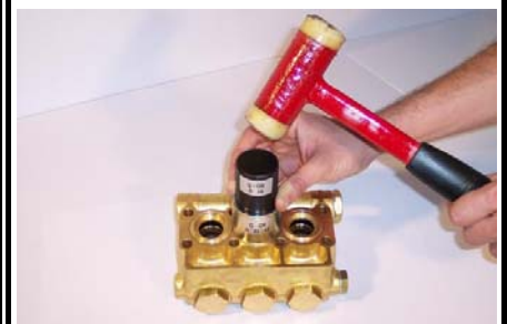
Push the pad in the bushing guide with the help of a rubber-faced hammer
