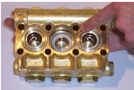
Push the spacer in the plunger's seat
