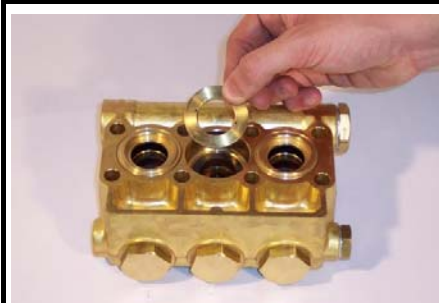
Insert the front brass ring in the plunger's seat
