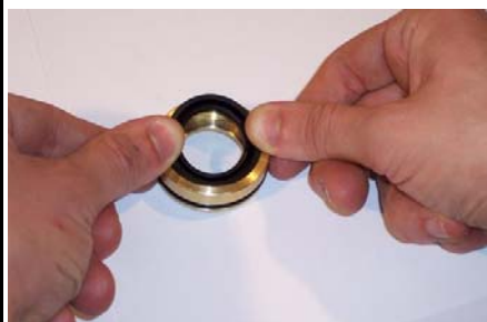
Push the back seal ring (the black one) in the back brass ring
