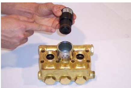
Place the front seal ring (the brown one) on the pad
