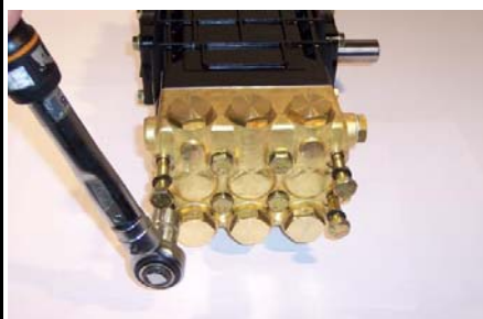
Turn the screws in, beginning from the middle ones (for torque specifications look at pages 10-11 of Operating Instructions Manual for Plunger Pumps)
